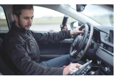
The **DrivingRobot** is also characterized by its compact design that frees up space and enables quick and hassle-free installation. The steering and throttle/brake robots are interconnected to provide ample room for electronics and data acquisition systems as well as easy access for test engineers. In addition, the **DrivingRobot** Box, contains all electronic components, which can be easily installed with ISOFIX in the rear seats
