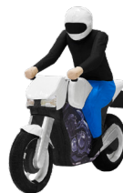
European Motorcycle Target & Stands 1 (UFO-1-5140) Euro NCAP approved with UFOnano
