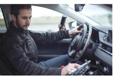
The DrivingRobot is also characterized by its compact design that frees up space and enables quick and hassle-free installation. The steering and throttle/brake robots are interconnected to provide ample room for electronics and data acquisition systems as well as easy access for test engineers. In addition, the all-inclusive DrivingRobot Box, containing all electronic components, can be easily installed with ISOFIX in the rear seat into the trunk.
