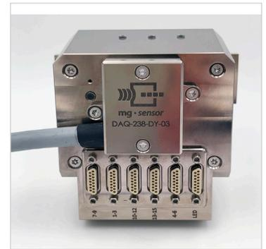
mg-sensor and the DTI solutions are accepted by Euro NCAP and compliant to all common standards like SAE J211 and ISO 6487. These standards specify basic features like filter, frequency response, sampling rates, A/D resolution, CFCs, CAC, accuracy, to ensure repeatable, reliable results.
