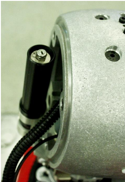
Figure 4.13 Rear Spring Adjustment Locknut Location
