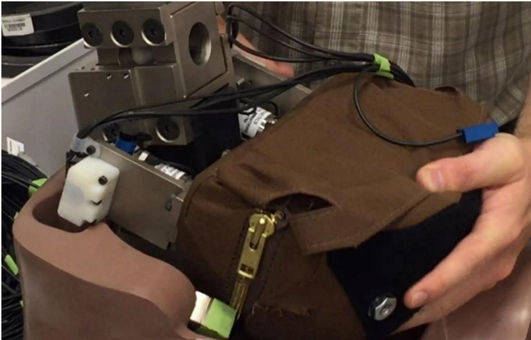
Figure 12.16 Insertion of Lower Abdomen into Dummy
