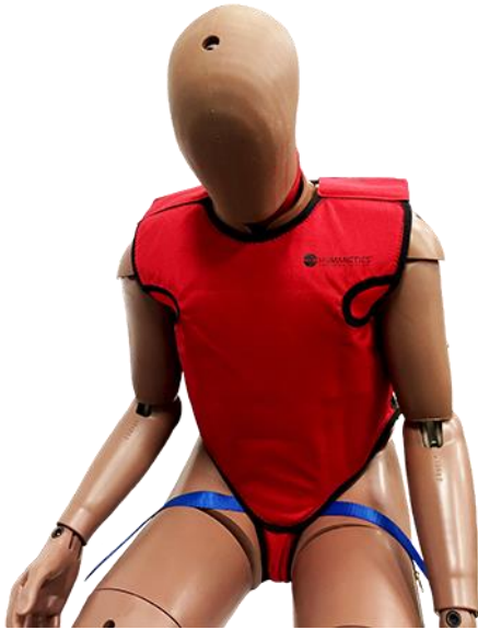
Figure 16.9 Properly Installed Jacket, Front
