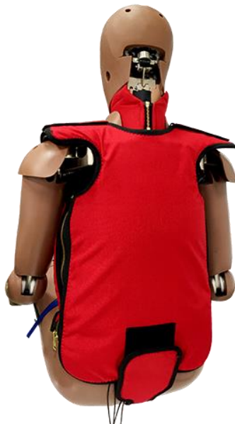
Figure 16.10 Properly Installed Jacket Assembly, Rear
