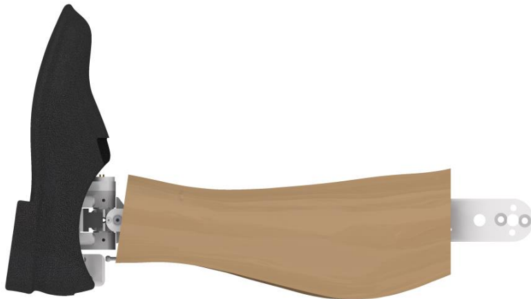
Figure 15.15 Completed THOR-LX Foot, Ankle and Lower Leg Assembly
