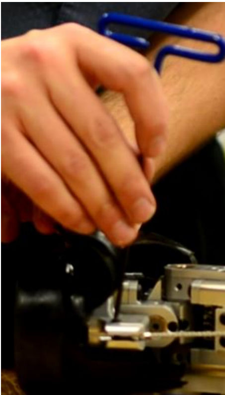
Figure 15.12 Secure Cable with Locking Screw
