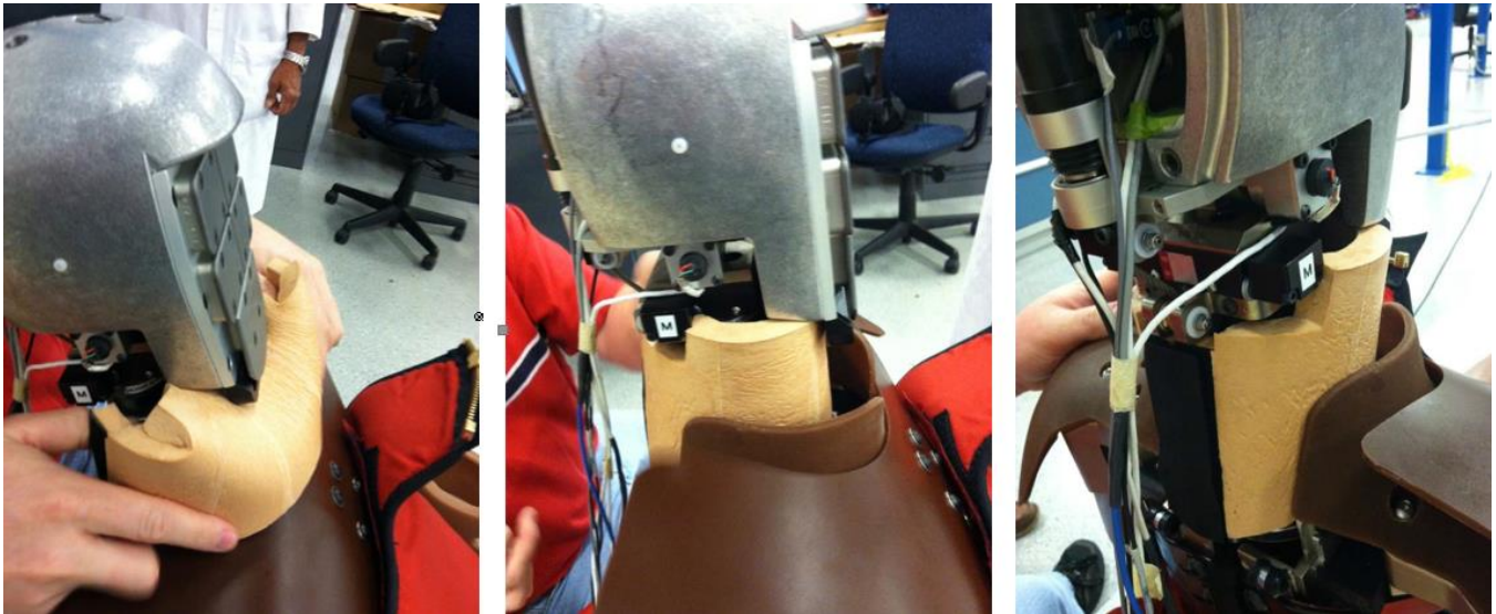
Figure 6.30 Slide Neck Foam Assembly under Chin
