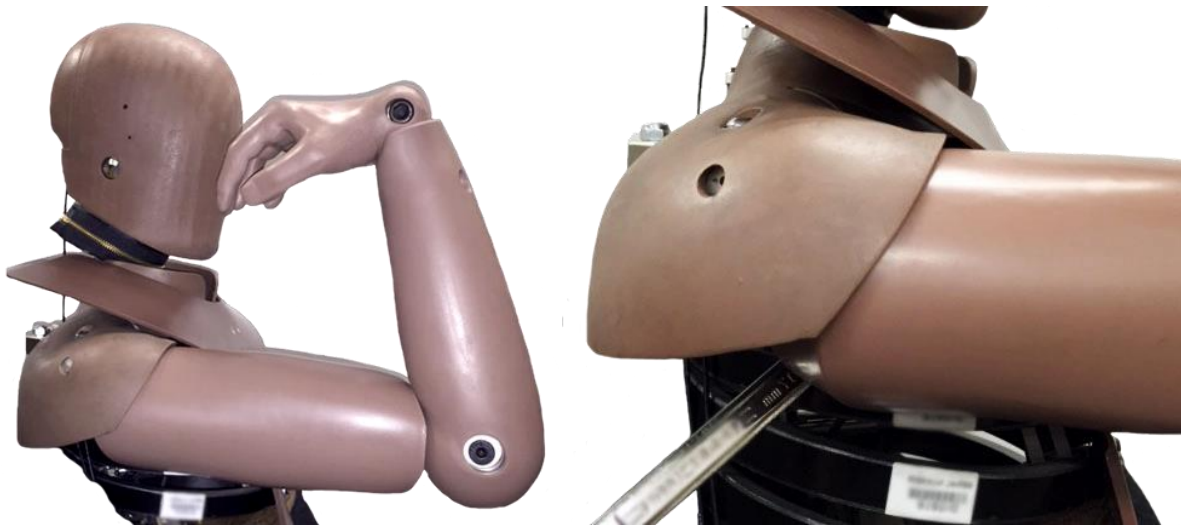
Figure 8.38 Upper Arm Y-Axis Adjustment
