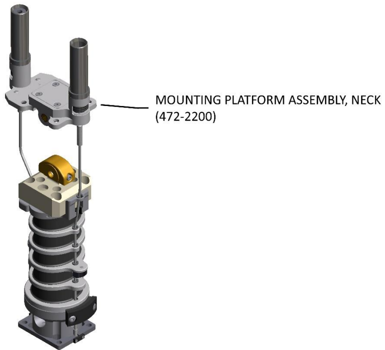
Figure 6.18 Neck Mounting Platform Assembly
