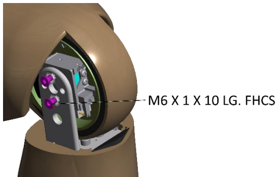
Figure 14.21 Knee Clevis to Kneecap Assembly
