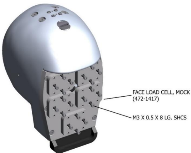
Figure 5.4 Assemble Face Load Cells
