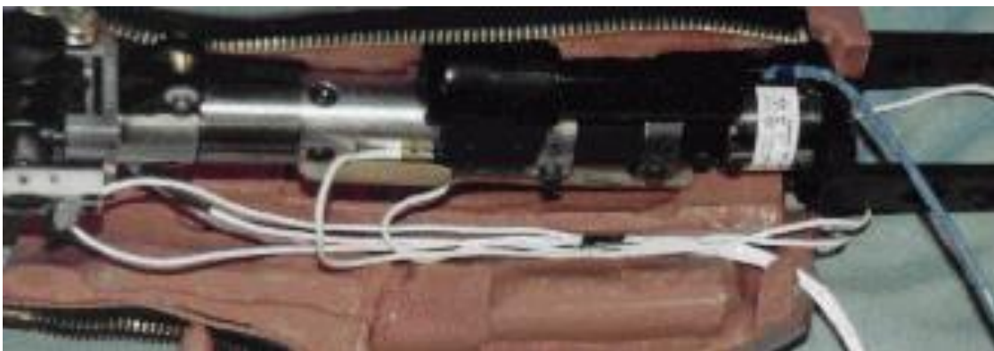
Figure 15.14 Route the Wiring in Lower Leg Skin
