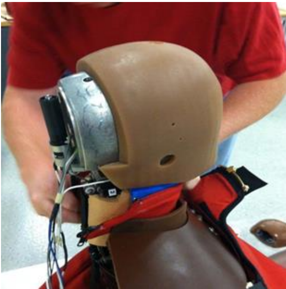
Figure 6.32 Tuck the Neck Skin Assembly Behind Shoulder Pads
