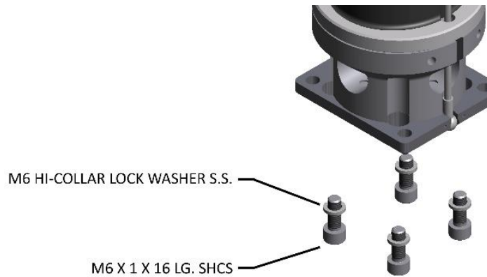
Figure 6.5 Secure Lower Neck LC with M6x16 SHCS and M6 Collar Lock Washer
