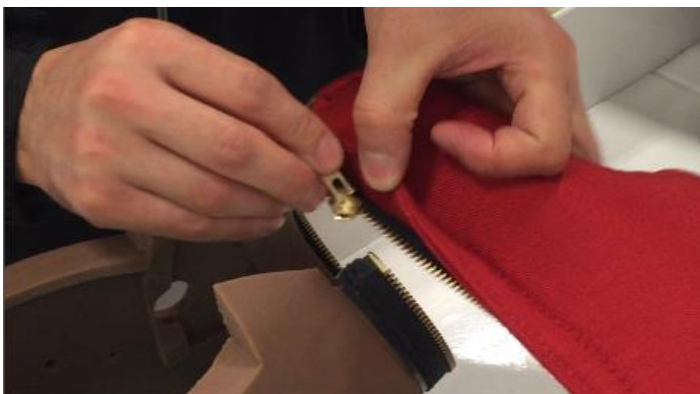
Figure 6.31 Zip Neck Foam Assembly to Head Skin
