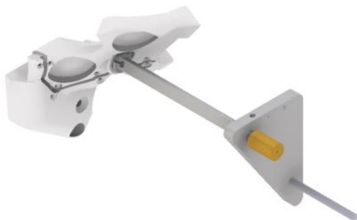
Figure 2.4 H-Point Tool Attached to Iliac
