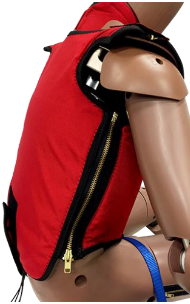
Figure 16.4 Jacket Assembled onto Thorax
