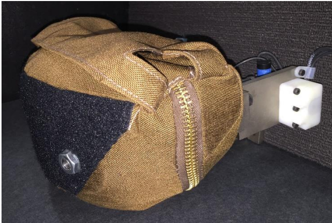
Figure 12.14 Completed Lower Abdomen Assembly
