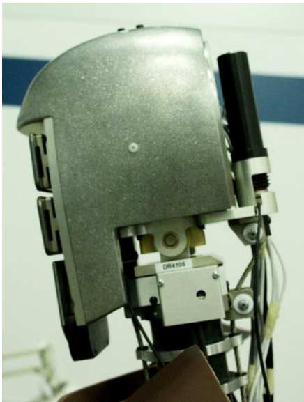
Figure 4.11 CG Marker Location on Head
