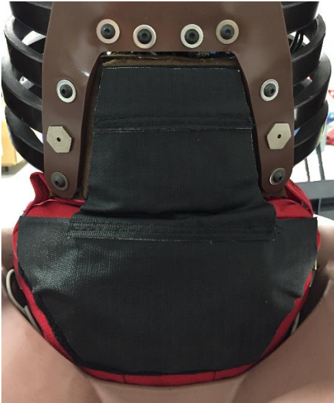
Figure 11.13 Proper Location of Upper and Lower Abdomen Cover
