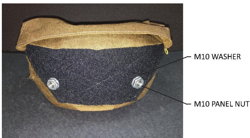
Figure 12.13 Securing of Nut and Washer to Outside of Bag
