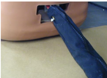
Figure 17.2 Mesh Cover Properly Positioned
