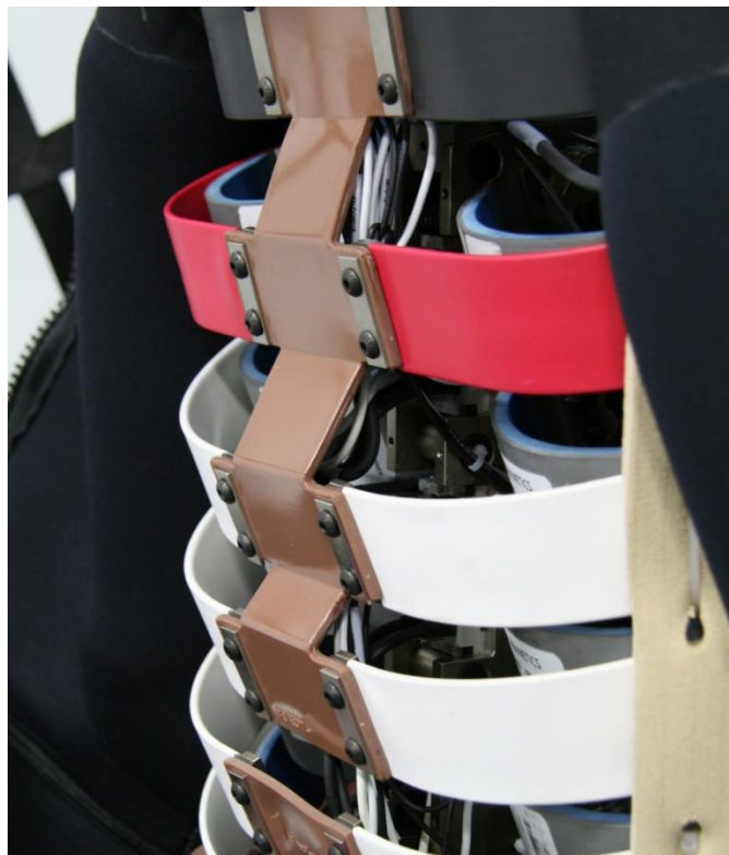
Figure 3-33 Rib instrumentation cables routed in the front to the DAS modules mounted in the spine box.
