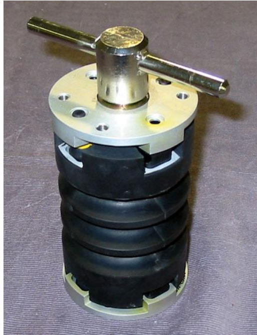
Figure 2-4 Using clamp to remove neck interface plate.
