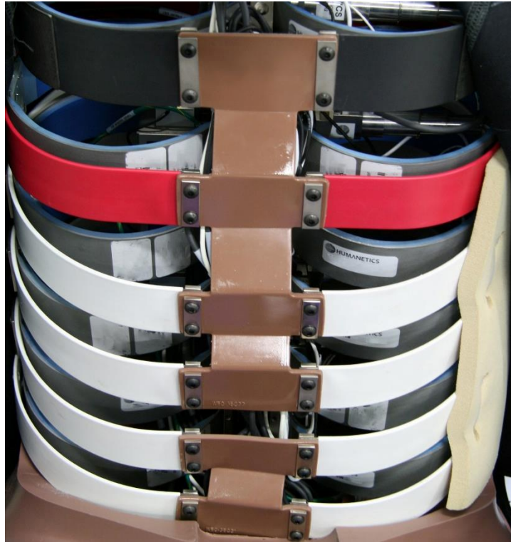
Figure 3-44 The sternum, thorax bib and abdominal rib coupler are attached to the ribs after instrumentation is plugged in.
