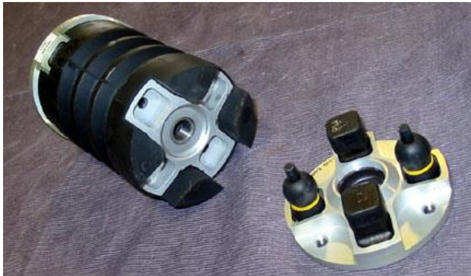
Figure 2-5 Neck buffers are free to remove when interface plates are removed.
