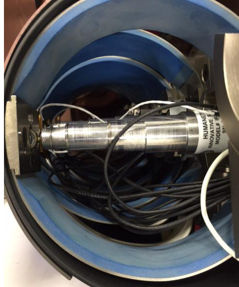
Figure 3-32 Wiring routing for rib instrumentation.
