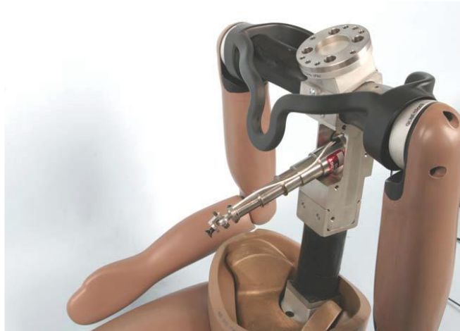
Figure 15. IR-TRACC should swing freely
