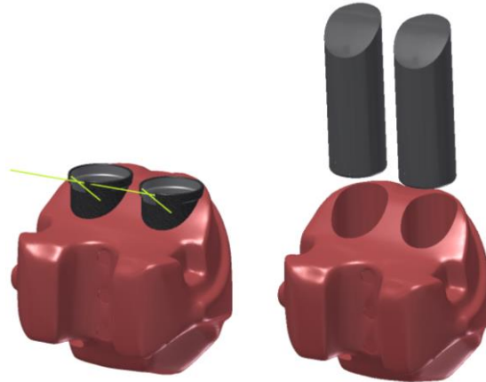
Figure 10. CAD Picture of Q6 Abdomen showing ATPS sleeves assembled without sensors and with foam plugs for certification
