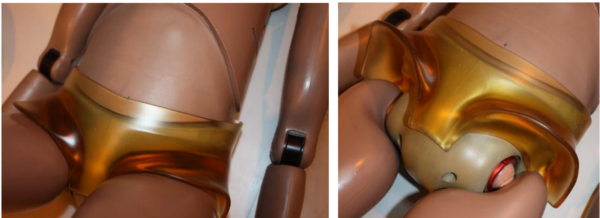
Figure 21. Hip insert fitted on Q-dummy: sitting position (left), straight legs (right)
