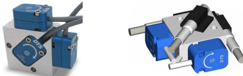
Figure 7. DTS ARS's on the special mount (IT-900)
