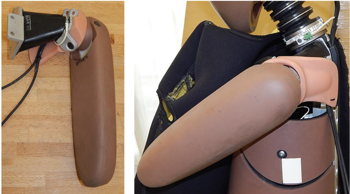
Figure 37. Q10 Side Impact Kit with shoulder joint accelerometer Ay (left) and T1 Ay accelerometers installed
