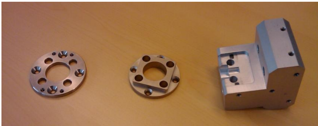
Figure 60. Picture showing from the left, neck adaptor plate (TE-010-2015), head drop ballast TE-010-1007 and lumbar central block TE-010-2650-14
