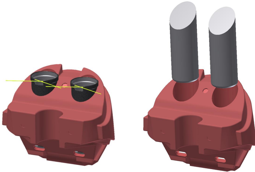
Figure 10. CAD Picture showing Q10 Abdomen APTS sleeves assembled without sensors and with foam plugs for certification
