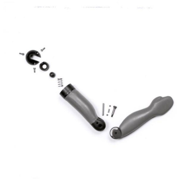
Figure 8: Disassembled (right) arm of the PI 1/2
