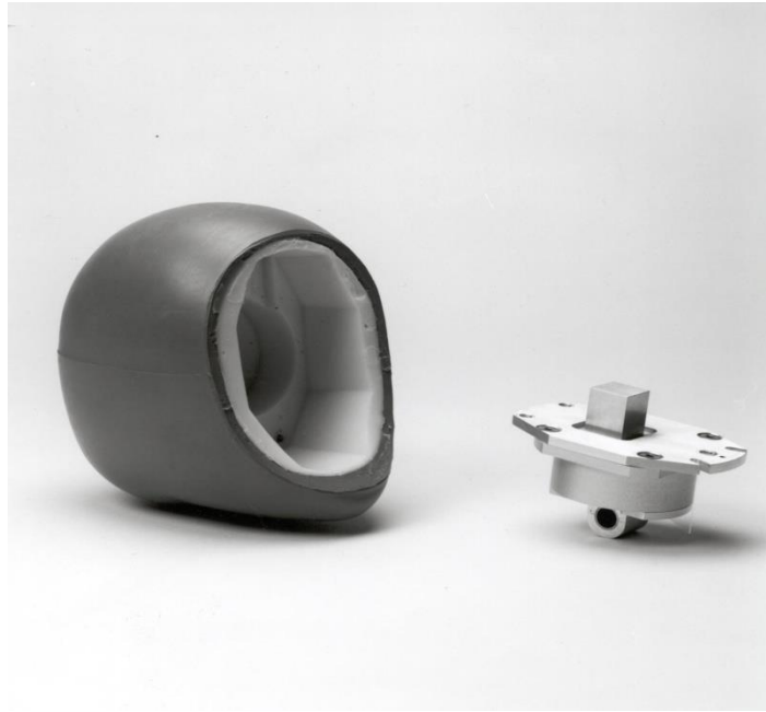
Figure 2: Parts of the head of the P1½: skull-skin moulding and other parts of the head in assembled state
