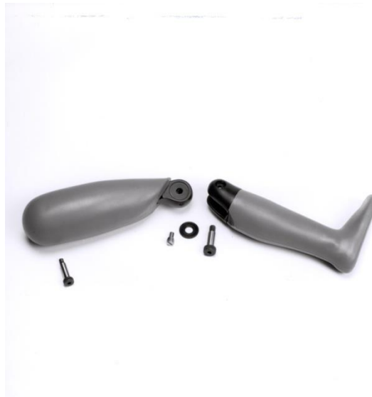
Figure 9: Disassembled (right) leg of the PI 1/2
