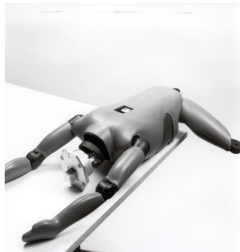
Figure 20: Hip abduction/adduction adjustment set-up
