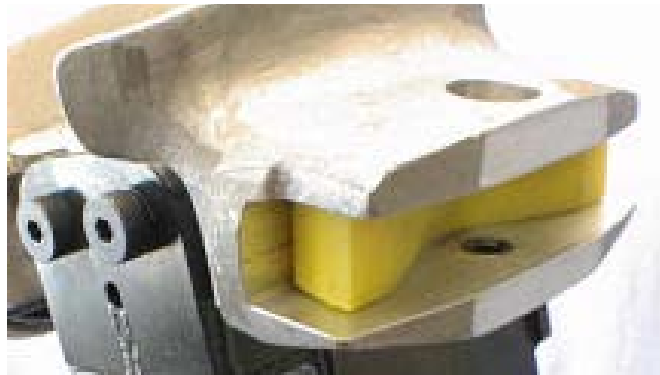
Figure 5.2.3.10: Location of urethane spring stop
