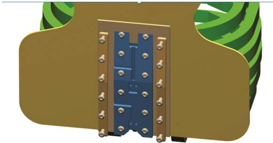
Figure 5.2.5.1: Removal of the BHCS fasteners holding the front of the ribs to the bib
