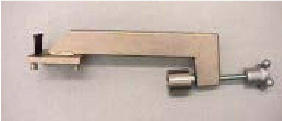
Figure 3.2.3.5: The neck compression tool
