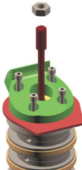
Figure 3.2.3.2: Removing the neck cable nut and fasteners
