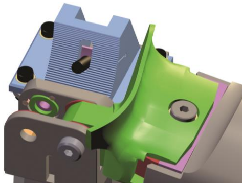
Figure 7.1.9.1: Installing clavicular link nuts and urethane washer nuts
