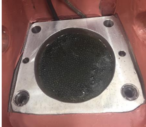
Figure 8.1.5.3: Potted lead shot (ballast) in cavity on top of pelvis
