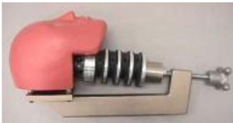
Figure 6.2.3.4: Neck compression tool installed on head and neck assembly
