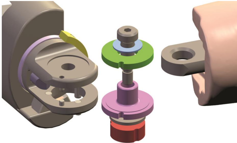
Figure 9.1.3.2: Exploded view of the shoulder yoke assembly
