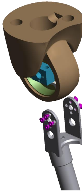
Figure 10.2.4.1: Detaching the lower leg from the knee
