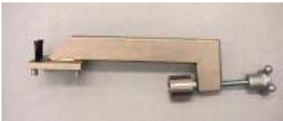
Figure 6.2.3.3: Neck compression tool
