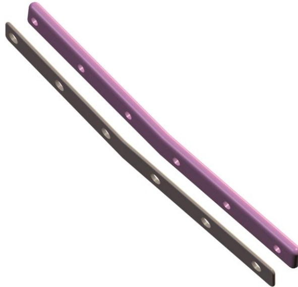
Figure 7.1.6.1: Thick and thin rib stiffeners at the bib
