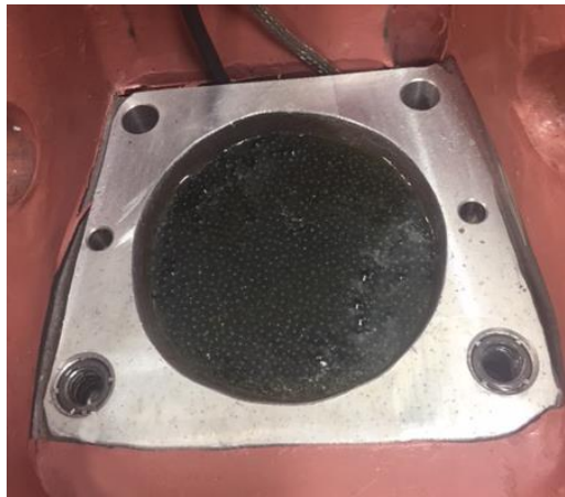
Figure 8.1.6.3: Potted lead shot (ballast) in cavity on top of pelvis
