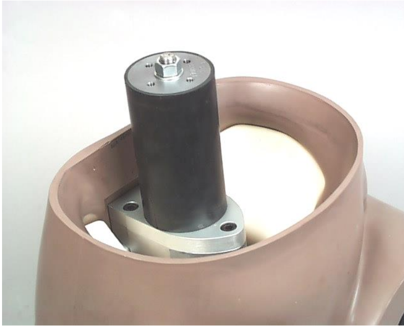
Figure 52: ES-2 lumbar spine and bottom plate mounted on pelvis assembly
