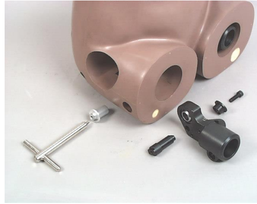
Figure 57: ES-2 pelvis, transducer bush and upper femur removed
