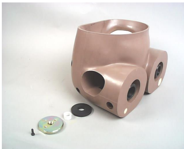
Figure 56: ES2 H-point back plate and its buffer assembly removed
