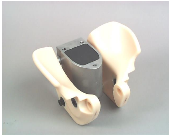
Figure 58: ES-2 pelvis internal parts sacrum block and iliac wings
