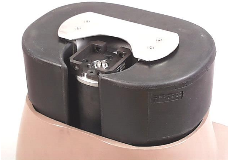
Figure 10: ES-2 abdomen seen from the back (dummy upper part removed)
