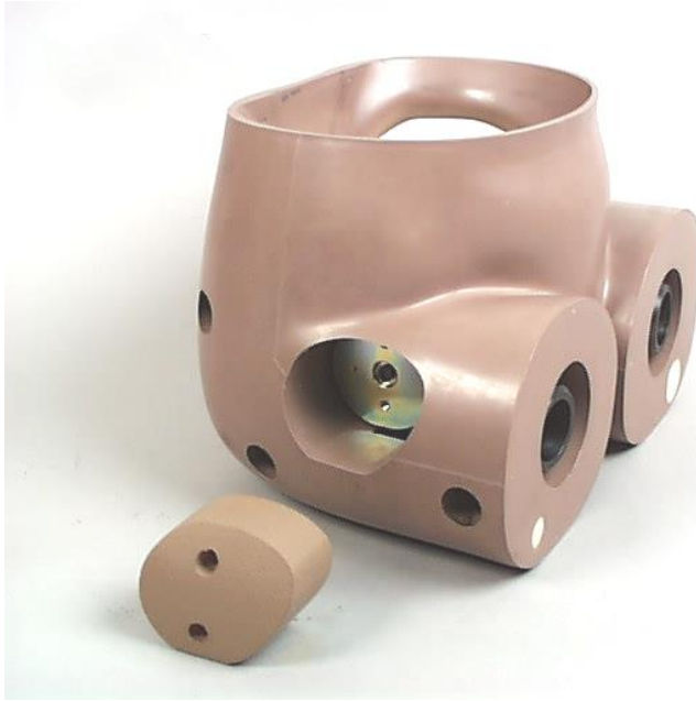
Figure 53: ES-2 pelvis with H-point foam block removed showing H-point back plate
