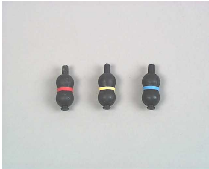
Figure 37: ES-2 neck circular section buffers. Three hardness' 60 (red), 70 (yellow) and 80 Shore A (blue)
