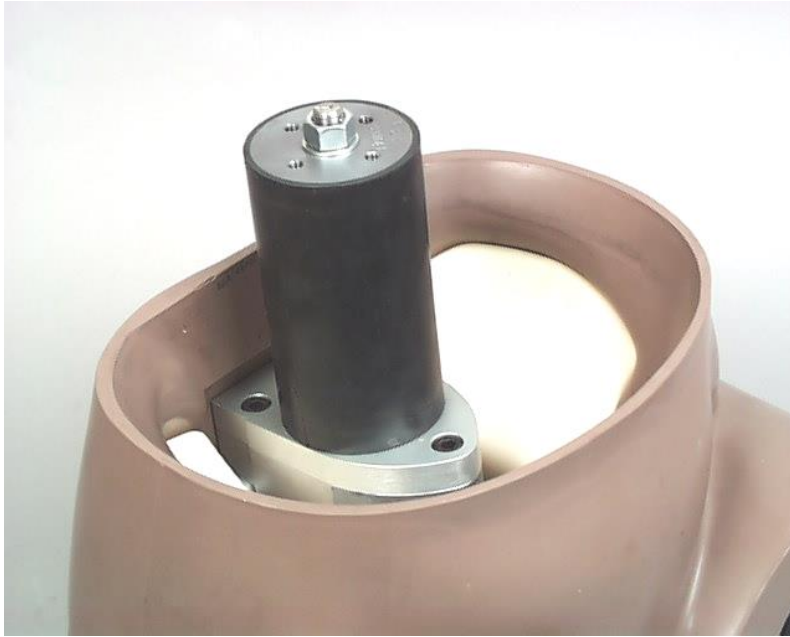
Figure 11: ES-2 lumbar spine (after removal of abdomen assembly)
