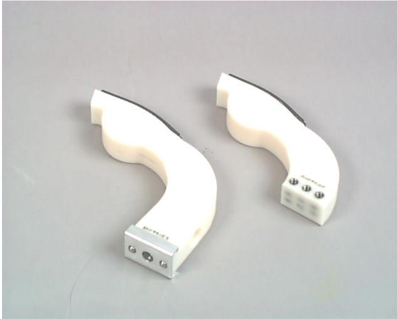
Figure 6: ES-2 standard clavicle and shortened clavicle for load cell installation (optional)
