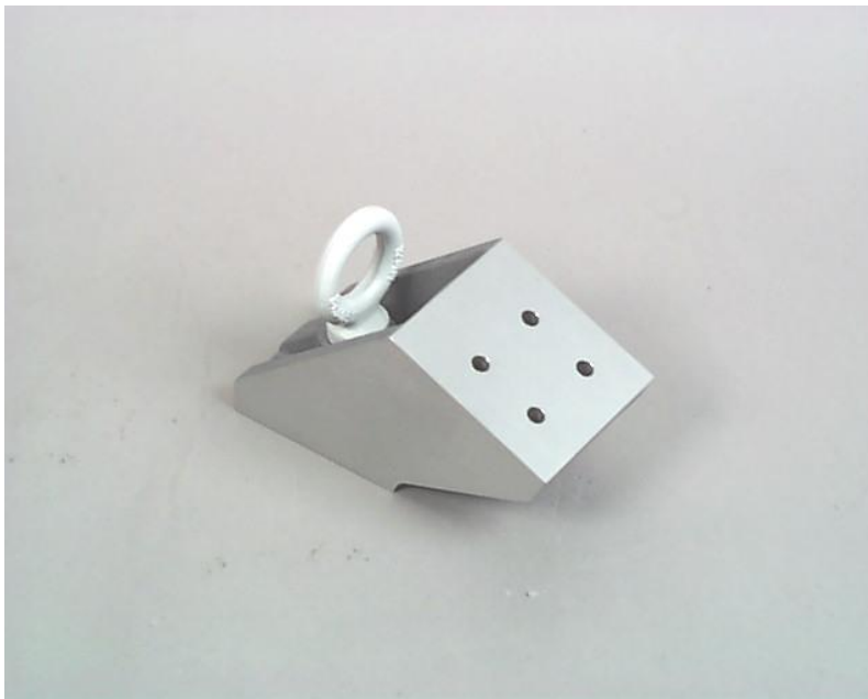
Figure 74: ES-2 lifting device – eyebolt in the neck bracket
