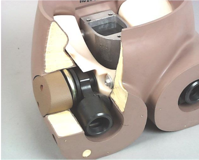
Figure 12: ES-2 pelvis (Foam partly cut away to show the hip joint. Lumbar mounting plate not shown)
