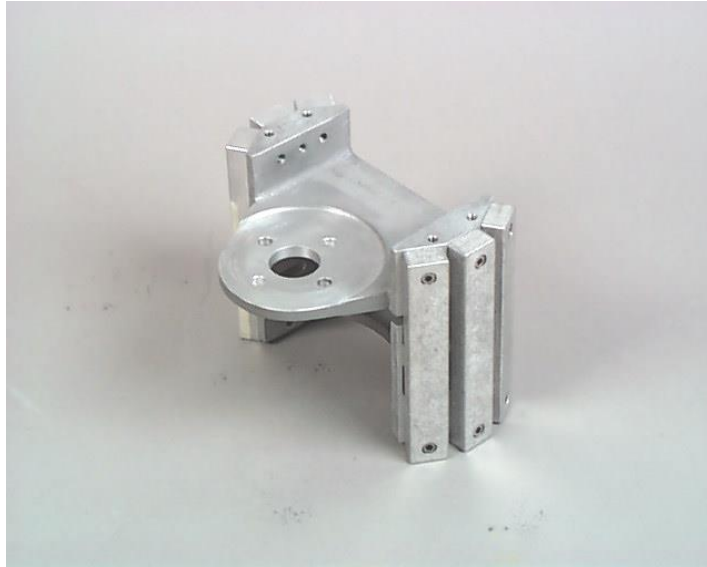
Figure 50: ES-2 abdomen drum and force transducer structural replacements
