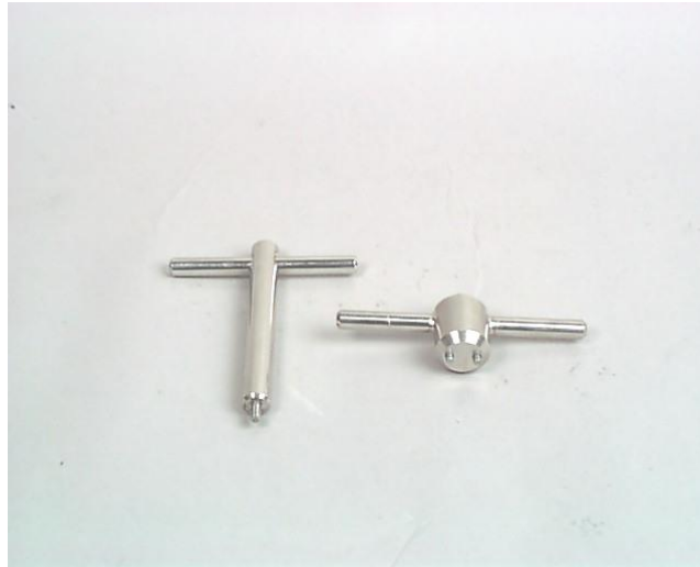
Figure 34: ES-2 pelvis puller tool (left) and neck compression tool (right)
