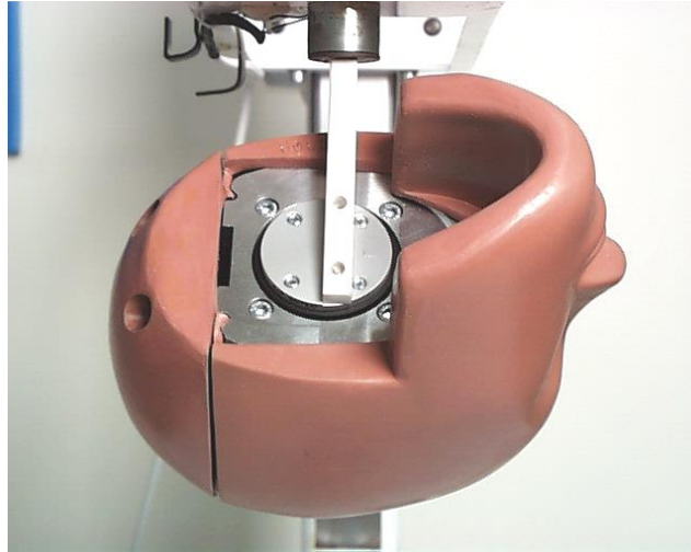
Figure 65: ES-2 head support bracket installed on the head (note the orientation)
