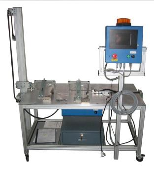
the added flexibility of performing tests in "manual" mode to allow the operator to move the upper torso through its range of motion, or to any position, and view transducer outputs throughout the entire range of motion. Analog outputs for the force and angle are provided on the bottom of the controller so that data can be collected by the user's DAS and software.
