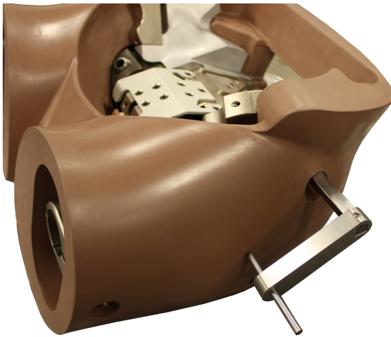
Figure 3 -New H-Point tool used to measure pelvis angle in conjunction with the new iliac wing design.
