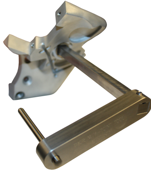
Figure 4 -New H-Point tool mounted in new iliac wing design.
