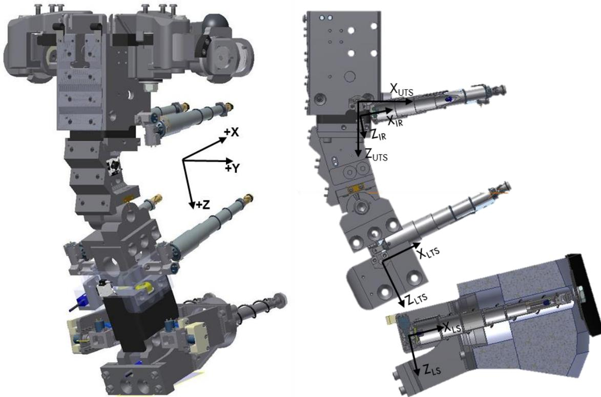
Figure 2: Global dummy coordinate system (left) and Local Spine Coordinate Systems seen on the right side of the dummy (right)
