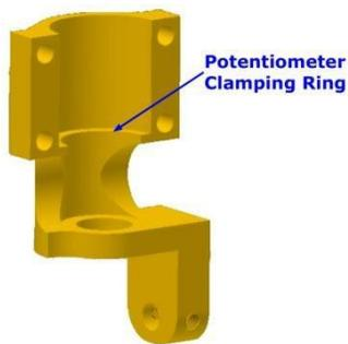
**Figure 8:** Mounting Bracket 472-3552 (Upper Left and Lower Right)
