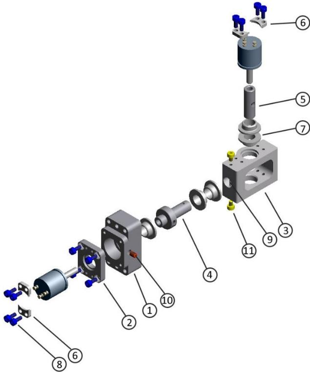
Figure 11: Exploded view of 472-4740-1 Left Abdominal Pivot Assembly.
