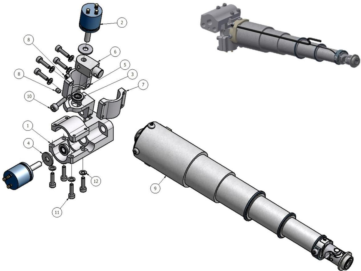
Figure 4: 472-3550 Upper Left Assembly (non-exploded: orientation mounted in the dummy)
