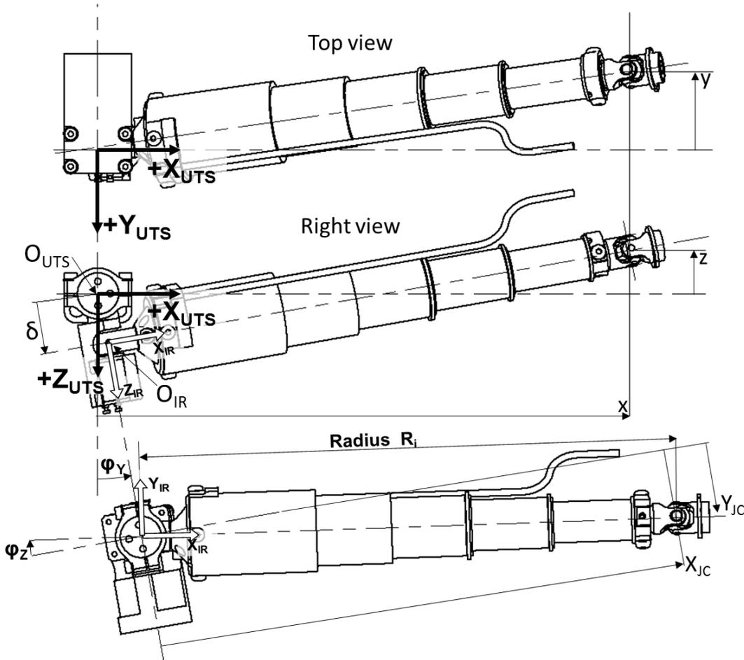
**Figure 25:** Upper Right 3D IR-TRACC top view in  $+Z_{UTS}$  direction, right view in  $-Y_{UTS}$  direction and bottom view on Z-axis angle sensor  $-Z_{IR}$ . The orientation of the 3D IR-TRACC corresponds roughly to the assembly orientation inside the dummy. Note that the values for y, z and  $\phi_z$  in this figure are negative.
