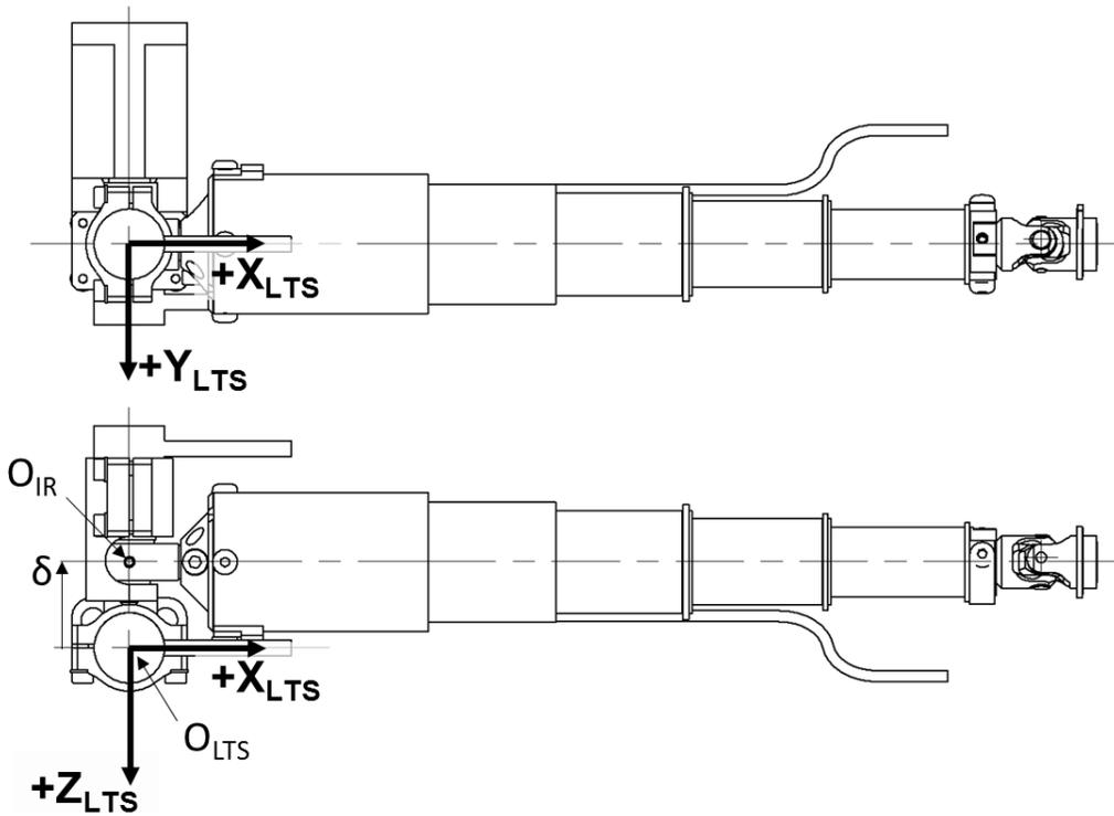
Figure 26: Lower Right 3D IR-TRACC top view in  $+Z_{LTS}$  direction, right view in  $-Y_{LTS}$  direction. The orientation of the 3D IR-TRACC corresponds roughly to the assembly orientation inside the dummy.
