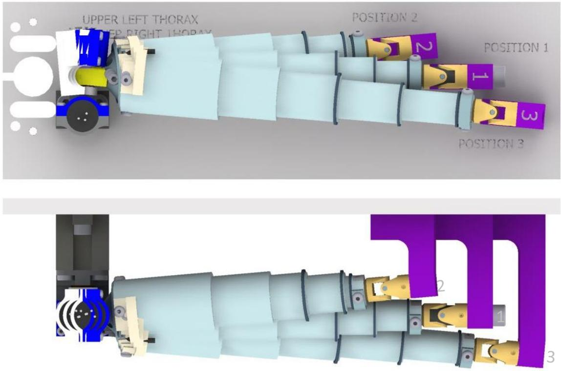
**Figure 15:** Upper Left Thorax IR-TRACC overlay; shown assembled at positions 1, 2, & 3 (view -Y direction above; +Z-direction below)
