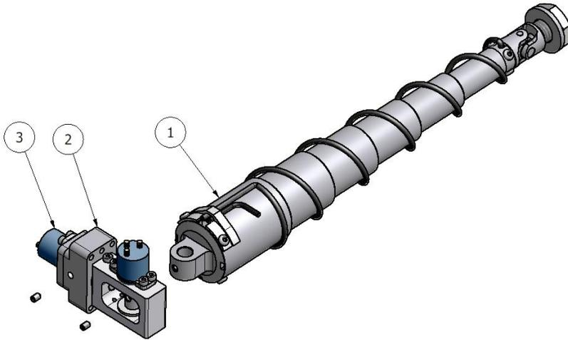
Figure 9: Exploded view of 472-4730-1 Left Abdominal 3D IR-TRACC Assembly
