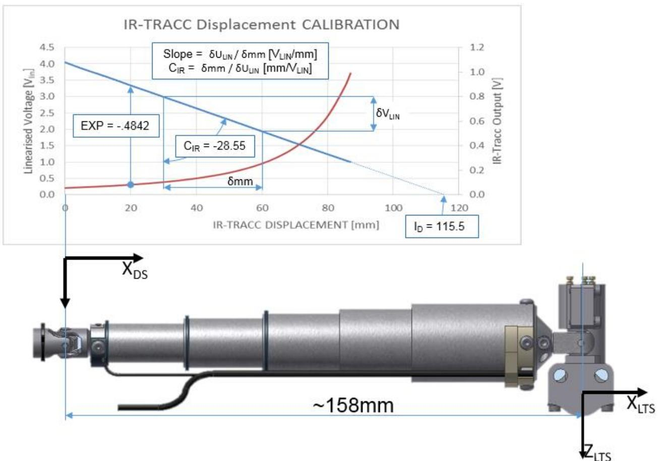
**Figure 28:** Displacement calibration example. Red line is nonlinear output of the IR-TRACC (scale right), blue line is the linearized output (scale left), including example parameters linearization exponent, calibration factor and displacement intercept. Note negative slope and mismatch of coordinate systems.
