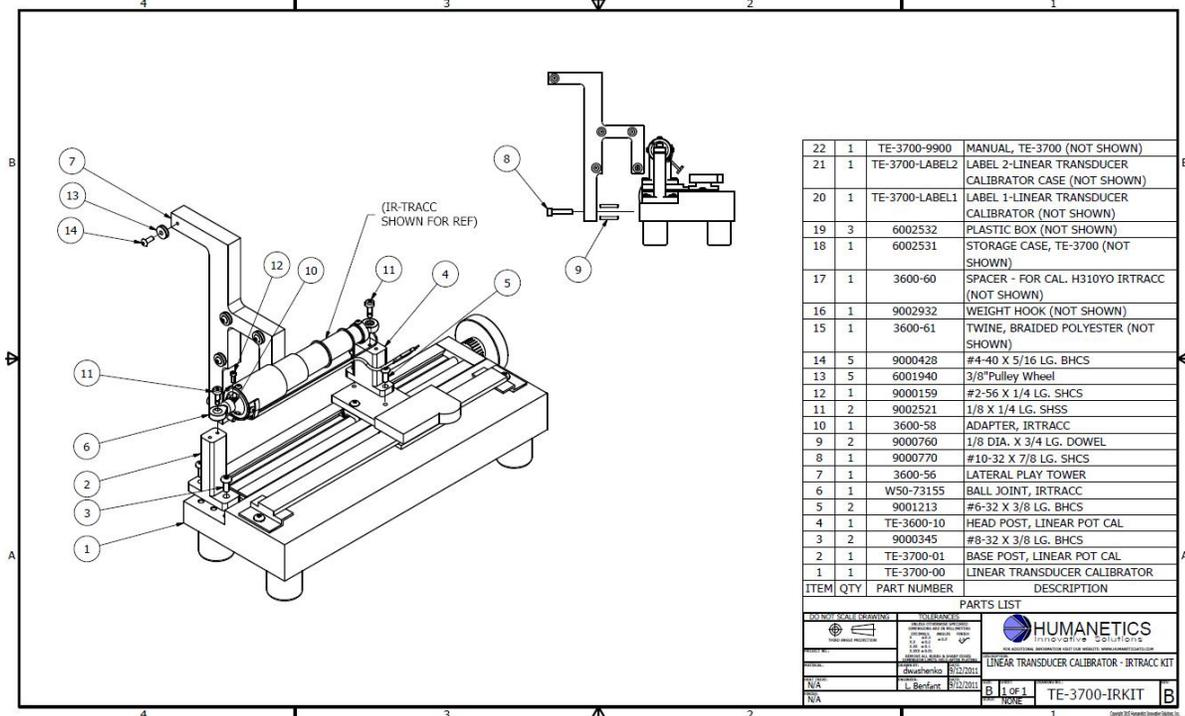
**Figure 13:** TE-3700-IRKIT, linear transducer calibrator
