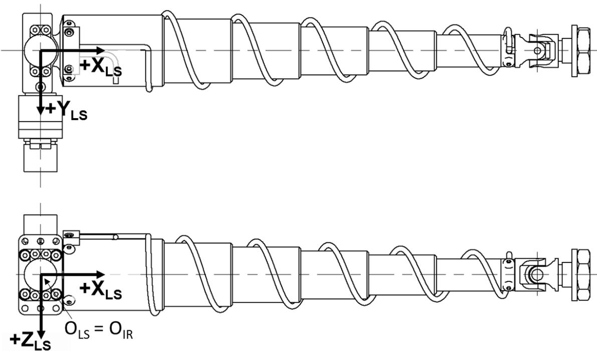
Figure 27: Right Abdomen 3D IR-TRACC top view in  $+Z_{LS}$  direction, right view in  $-Y_{LS}$  direction.
