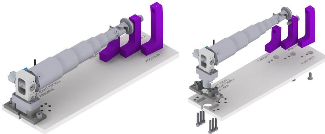
**Figure 20:** Left Abdomen 3D IR-TRACC assembly shown installed (left) and exploded (right). (Right abdomen assembly mounts to the opposite side of the base plate.)
