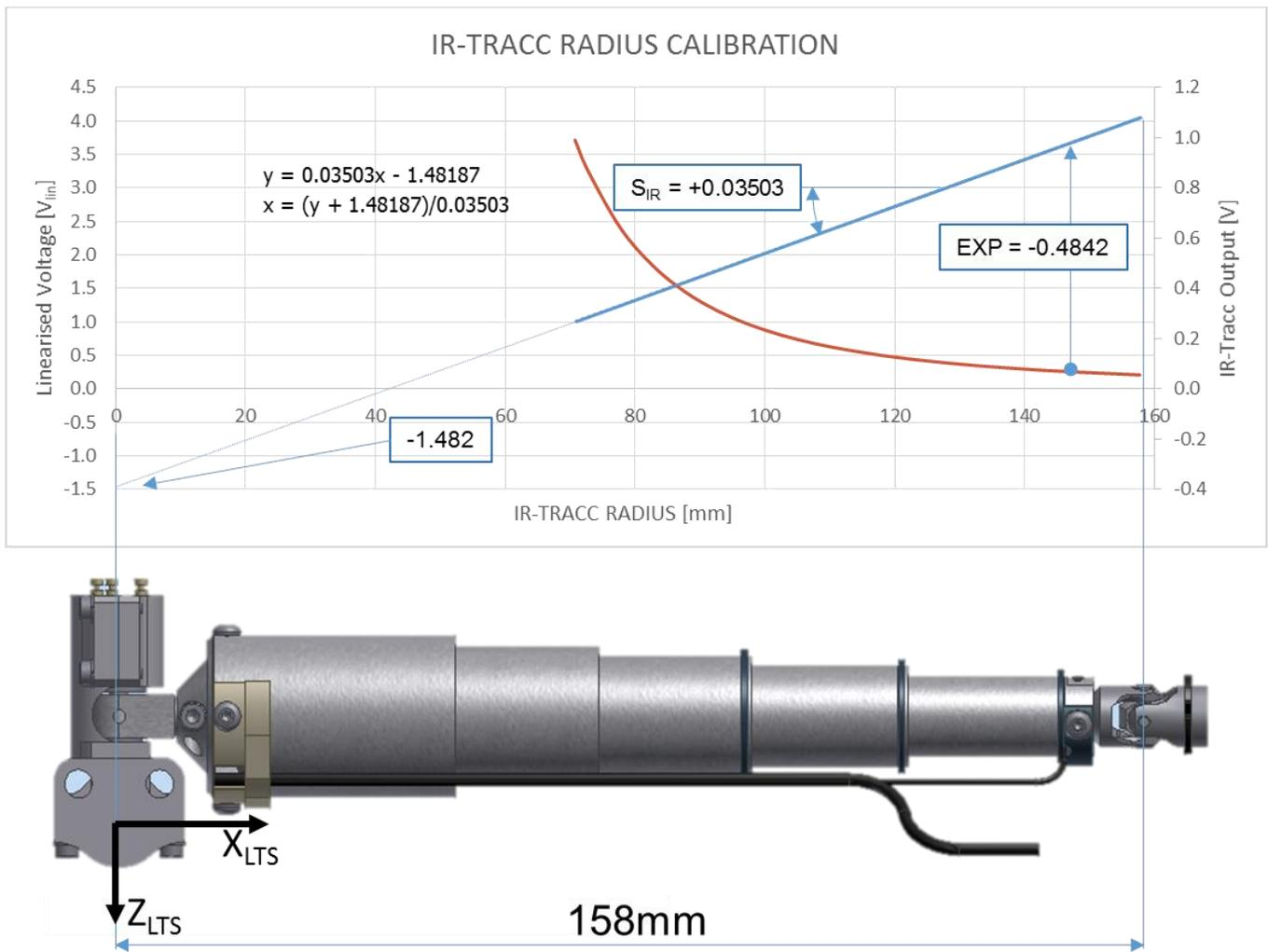
Figure 31: Calibration parameters expressed in Linearized Volts, same example IR-TRACC
