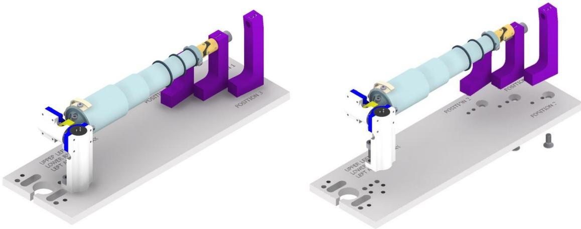
**Figure 19:** Lower Right Thorax 3D IR-TRACC assembly shown installed (left) and exploded (right). (Lower left assembly mounts to the opposite side of the base plate).
