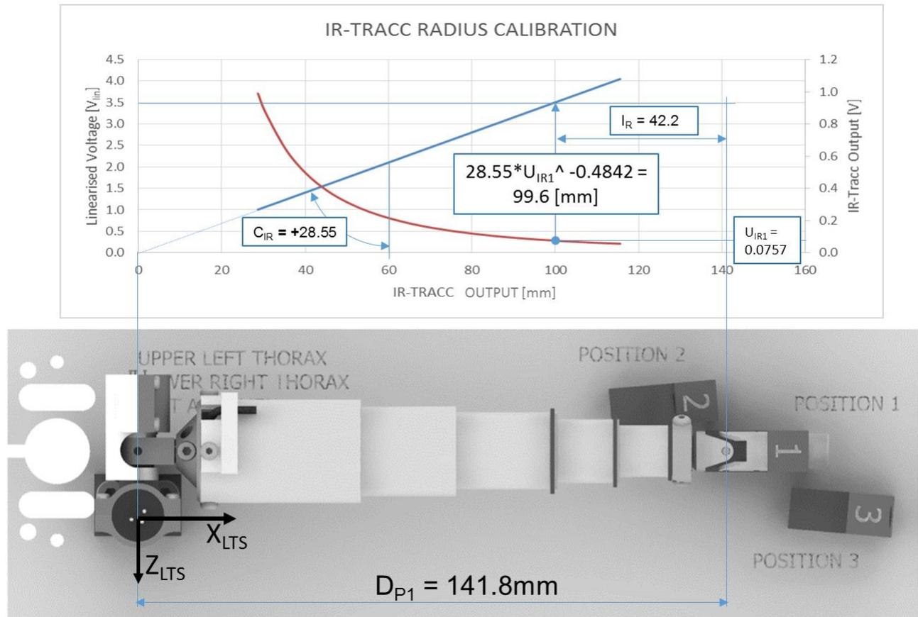
**Figure 29:** Calculation of Radius Intercept  $I_R$ . Red line is nonlinear output of the IR-TRACC (scale right), blue line is the linearized output (scale left), including example parameters.
