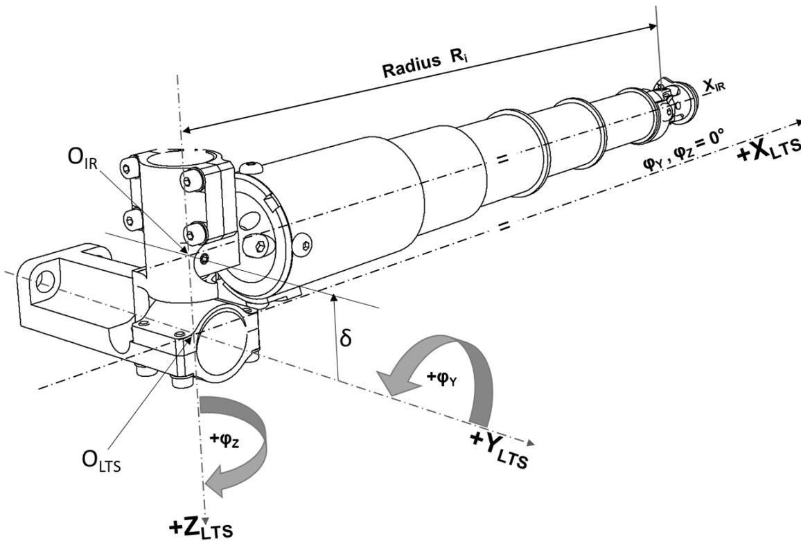
Figure 3: 3D IR-TRACC Lower Right aligned with LTS coordinate system (IR-TRACC axis parallel with X-axis)
