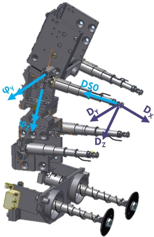
**Figure 1:** Six versions 3D IR-TRACCs in the THOR dummy
