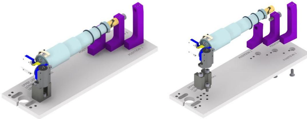
Figure 18: Upper Left Thorax 3D IR-TRACC assembly shown installed (left) and exploded (right). (Upper right assembly mounts to the opposite side of the base plate).
