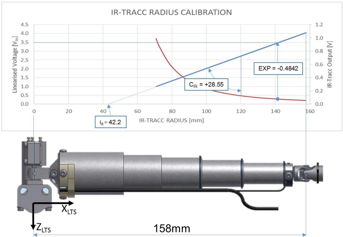
**Figure 30:** Calculation of IR-TRACC Radius from calibration parameters, including example parameters.
