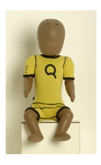
The Q0 child dummy is designed as a tool to evaluate the protection offered newborn children by appropriate child restraints used in cars as specified in the restraint manual for frontal, rear, side impact, and rollover crash conditions.
