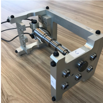
The new zero-position fixture shown with a typical IR-TRACC in the "ZERO" Position
