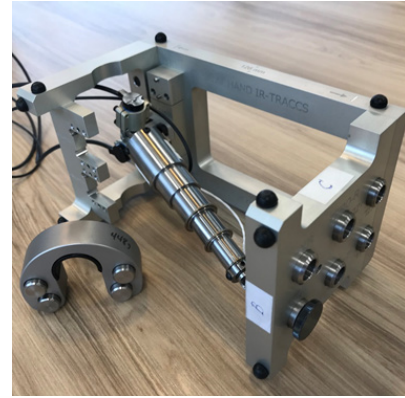
The new zero-position fixture shown with a typical IR-TRACC in the "+YZ" Position
