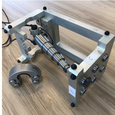
The new zero-position fixture shown with a typical IR-TRACC in the "+Y" Position
