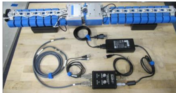
Figure 36 Leg with disconnect wire, TDAS interface and power supply
