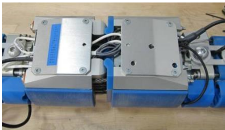
Figure 34 LH of leg with knee covers fitted 12 channels. Leg wires are not shown secured.
