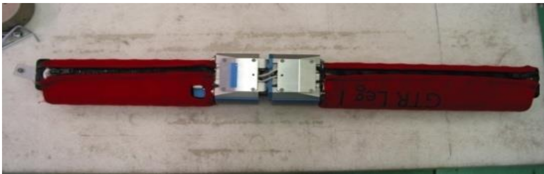
Figure 71 Assembly of first flesh layer
