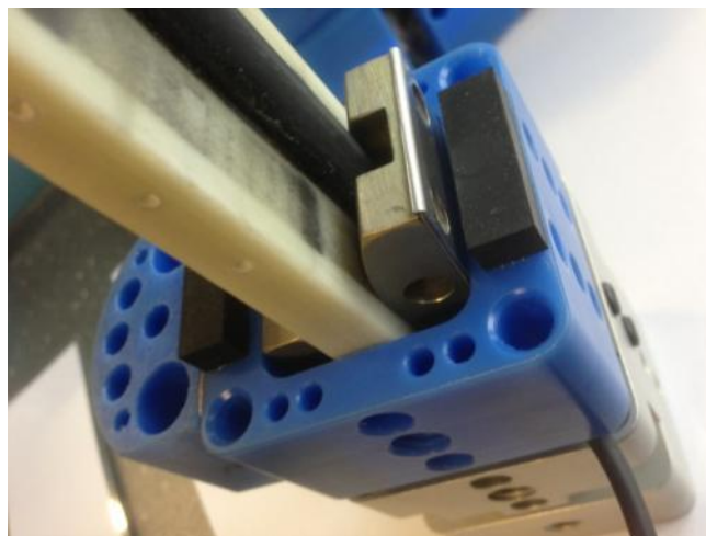
Figure 59 Fitting thin bone spacer with captive shim
