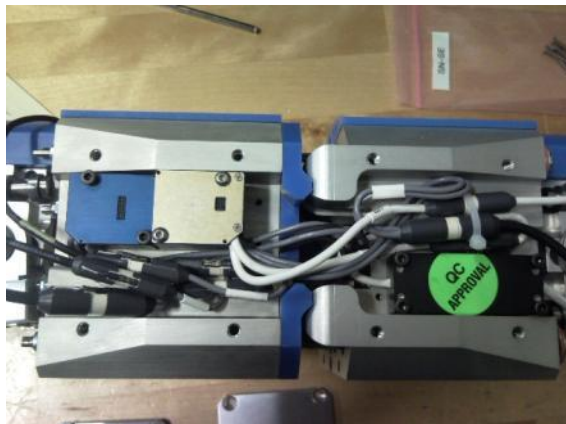
Figure 38 Left side wiring example of 24 channel SLICE
