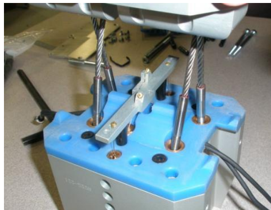
Figure 66 Cross wire feed through on knee
