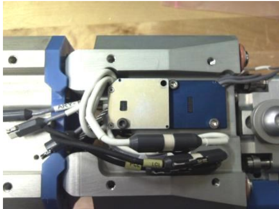
Figure 37 Optional SLICE unit 24 channel option (right side)
