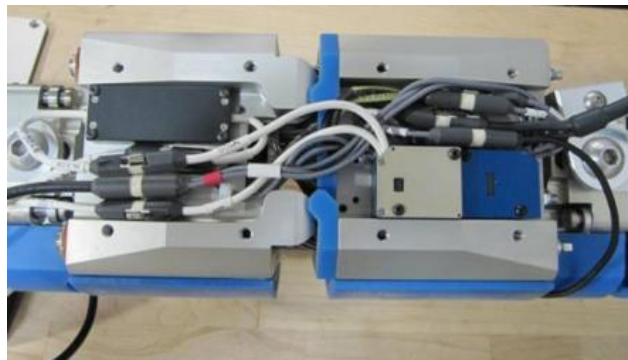
Figure 32 Typical 12 channel Slice wiring to knee
