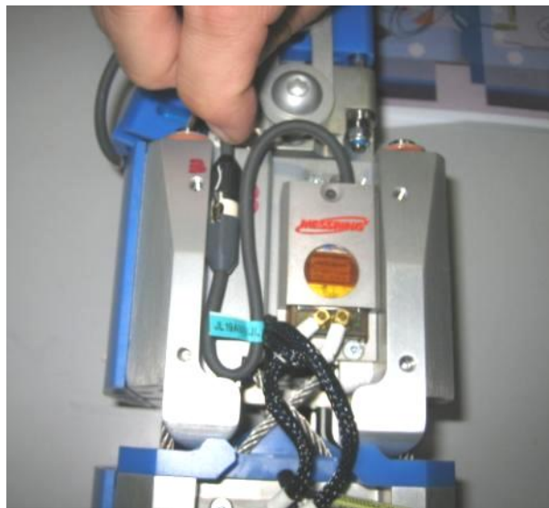
Figure 29 Top left-hand side of knee Messring 24 channels sensors connected
