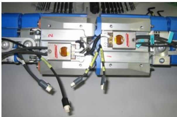
Figure 26 Right hand side of knee M=BUS 24 channels, sensors not connected
