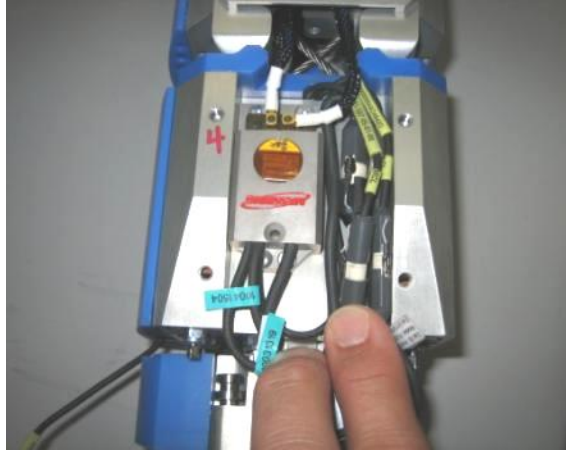
Figure 30 Bottom left-hand side of knee M=BUS 24 channels, sensors connected
