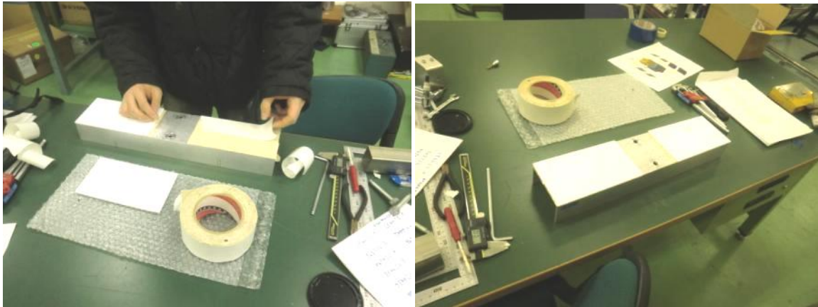
Figure 78 Example of fixing Teflon sheet to base plate
