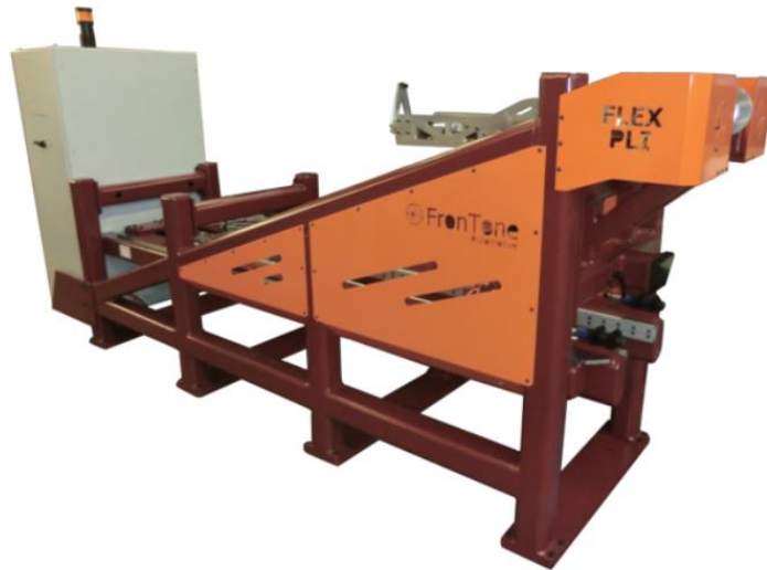
Figure 90 FLEX ZERT, pendulum arm folded back in inverse condition with control box
