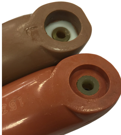
Fig. 1 - Harmonized upper arm (top) next to the Denton brand upper arm (bottom).
