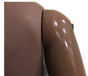
Fig. 2 - Harmonized upper arm flush to the CRABI torso jacket
