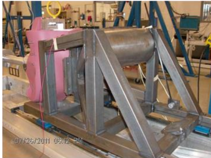
Figure 4: BioRID Jacket Sled Setup
