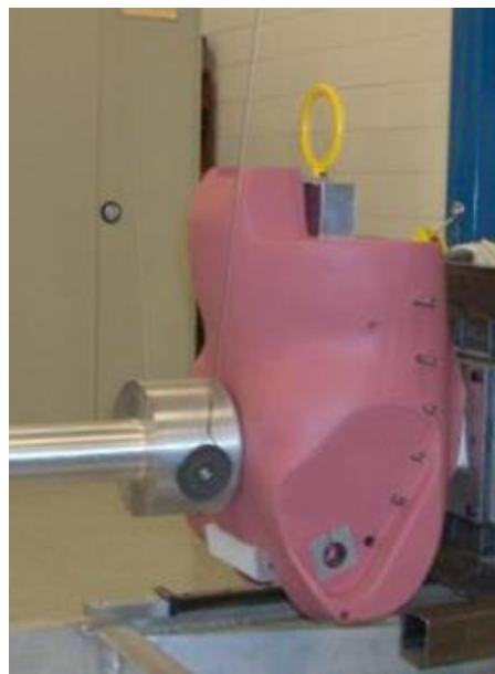
Figure 5: BioRID Jacket Test Setup
