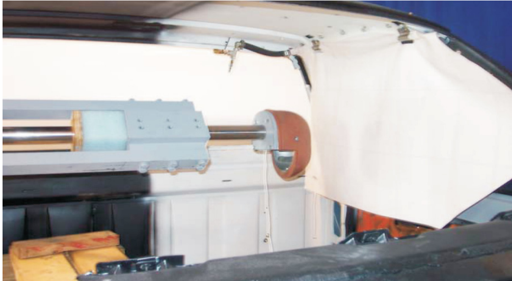
Figure 8. Headform Mounted on Impactor Photo courtesy of NHTSA
