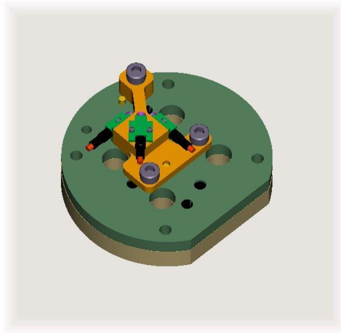
Figure 20: ES-2re Head Accelerometer Orientation on Structural Replacement
