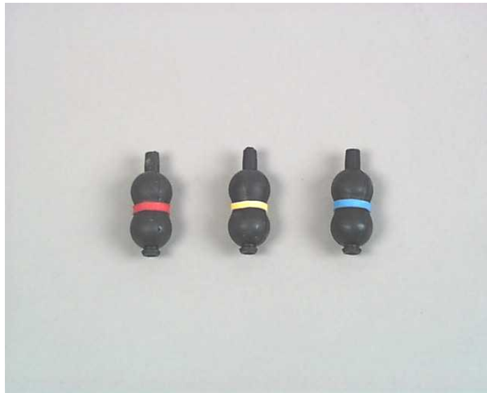
Figure 39: ES-2re Neck Circular Section Buffers Three Hardness Levels: 60 (Red), 70 (Yellow) and 80 (Blue) Shore A
