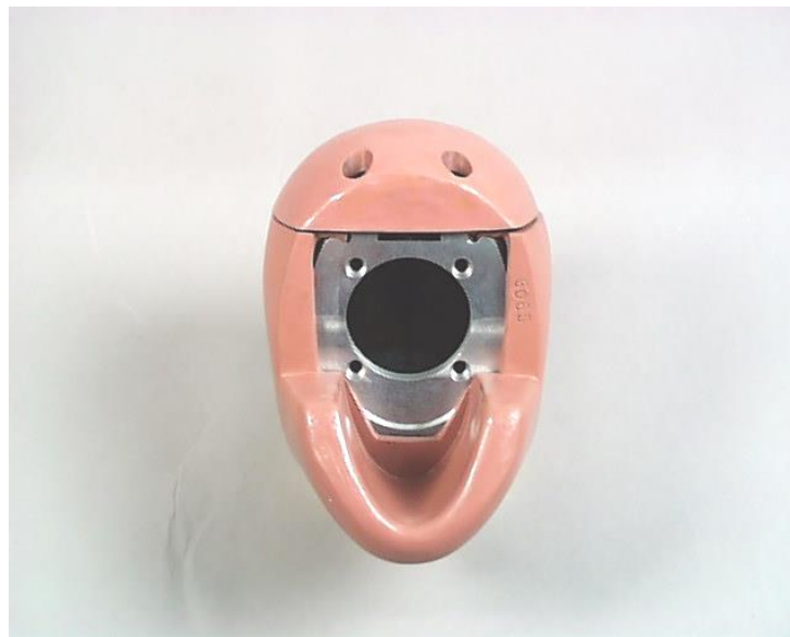
Figure 5: ES-2re Head Showing Interface
