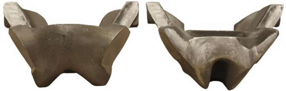
FTSS and Denton raw pelvis bone castings showing differences in shape
