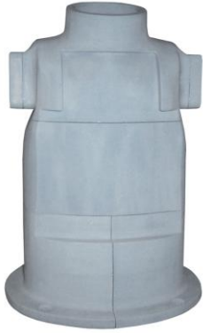
Mandrel used for inspecting the fit of the 2009 harmonized chest jacket
