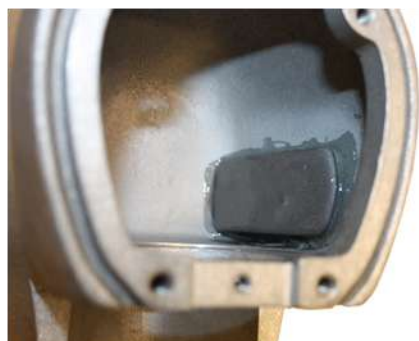
Ballast attached to interior of skull cavity
